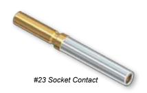
Standard size #23 contacts accept #22 to #28 AWG wire. Choose "small bore" versions for #26 to #30 AWG wire. For thermocouple applications, specify alumel or chromel contacts. Contacts are bulk packaged. Terminate with standard M22520 crimper with special positioner.
