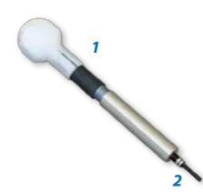
Check for properly seated contacts with this spring-loaded tester. Apply the tool tip to the mating end of a contact. Push on the handle until the spring compresses to the recommended force. A visual indicator shows full compression. The contact is properly retained if it is not displaced. The adjustable handle should be set to 3.2 pounds (14.2 N). The pin tip is used with #23 pin contacts. The socket tip is used with #23 socket contacts.
