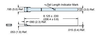
The 600-090 Extended Length Standard Band is precision constructed of 300 Series SST/Pas-
