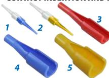
Install and remove PowerTrip $^{\text{m}}$  contacts with plastic tools. Size #12 and #16 tools are used for both insertion and extraction. Size 8, 4 and 1/0 tools are used for contact removal only.
