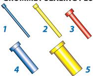
Grommet sealing plugs prevent moisture and contamination from entering unwired connector positions. Molded thermoplastic. Size 12 and size 16 plugs can be inserted with contact insertion tools. Size 8 and larger can be inserted by hand with no tool. Bulk packaged.
