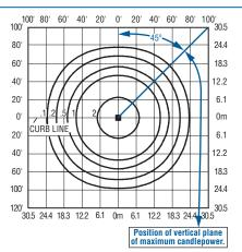
Isofootcandle plot of 4300K, 120 LED Type V Short area round luminaire at 25' (7.6m) A.F.G. Luminaire with 17,235 initial delivered lumens operating at 525mA. Initial FC at grade.
