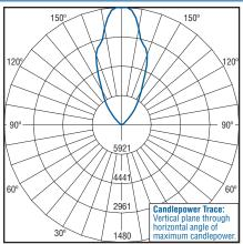
Independent Testing Laboratories certified test. Report No. ITL68434. Candlepower trace of 5700K, 2' (.6m) linear flood luminaire with 14 LEDs per foot. 40° flood optic with 4,588 initial delivered lumens operating at 700mA. All published luminaire photometric testing performed to IESNA LM-79-08 standards.
