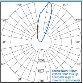
Independent Testing Laboratories certified test. Report No. ITL68433. Candlepower trace of 5700K, 2' (.6m) linear flood luminaire with 14 LEDs per foot. Sign Light optic with 4,506 initial delivered lumens operating at 770mA. All published luminaire photometric testing performed to IESNA LM-79-08 standards.
