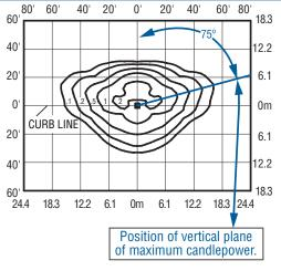
Independent Testing Laboratories certified test. Report No. ITL69283. Candlepower trace of 5700K, 2' (.6m) linear flood luminaire with 14 LEDs per foot. Type II Medium with 3,867 initial delivered lumens operating at 700mA. All published luminaire photometric testing performed to IESNA LM-79-08 standards.
