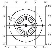
Isofootcandle plot of 4000K, 60 LED,  $15^{\rm o}$  flood EDGE round luminaire at 20' (6.1m) A.F.G. Luminaire with 10,668 initial delivered lumens operating at 700mA. Initial FC at grade.
