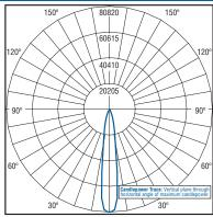
Independent Testing Laboratories certified test. Report No. ITL71408. Candlepower trace of a 4000K, 60 LED 15° flood optic flood EDGE round luminaire with 11,416 initial delivered lumens operating at 700mA. All published luminaire photometric testing performed to IESNA LM-79-08 standards.
