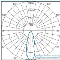
Independent Testing Laboratories certified test. Report No. ITL71498. Candlepower trace of a 4000K, 60 LED 25° flood optic flood EDGE round luminaire with 11,148 initial delivered lumens operating at 700mA. All published luminaire photometric testing performed to IESNA LM-79-08 standards.
