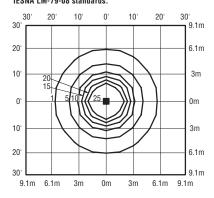
Isofootcandle plot of 4000K, 60 LED, 25° flood EDGE round luminaire at 20' (6.1m) A.F.G. Luminaire with 10,668 initial delivered lumens operating at 700mA. Initial FC at grade.
