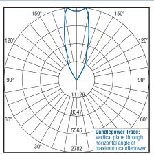
Independent Testing Laboratories certified test. Report No. ITL68425. Candlepower trace of 5700K, 2' (.6m) linear flood luminaire with 14 LEDs per foot. 25° flood optic with 5,132 initial delivered lumens operating at 700mA. All published luminaire photometric testing performed to IESNA LM-79-08 standards.
