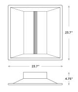
NOTE: Use of Expanded Junction Box will expand the depth to  $6.67^{\prime\prime}$  and Emergency Backup will expand the depth to  $6.30^{\prime\prime}$ .
