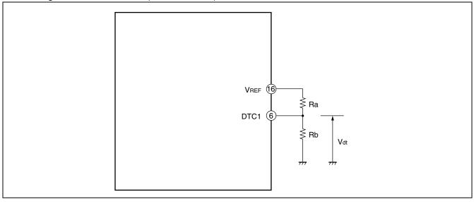
• Setting the idle time at DTC1 (DTC2 is similar)
