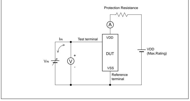
Note : The voltage V<sub>IN</sub> is increased gradually and the current IIN of 300 mA at maximum shall flow. Confirm the latch up does not occur under  $I_{IN} = \pm 300$  mA. In case the specific requirement is specified for I/O and  $I_{IN}$  cannot be 300 mA, the voltage shall be increased to the level that meets the specific requirement. • C-V method of Latch-Up Resistance Test
