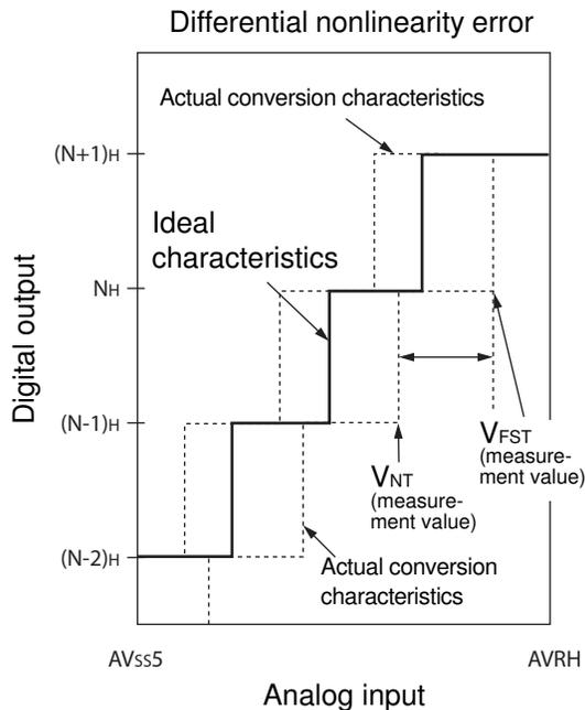
$$\text{Nonlinearity error of digital output } N = \frac{V_{NT} - \{1\text{LSB} \times (N - 1) + V_{OT}\}}{1\text{LSB}} \text{ [LSB]}$$
