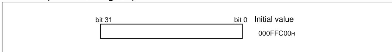
The table base register stores the starting address of the vector table used in EIT processing.
