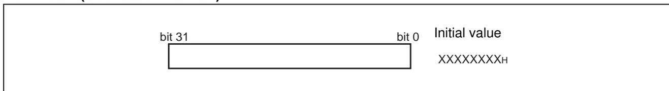
The user stack pointer, when the S flag is "1", this register functions as the R15 register.
