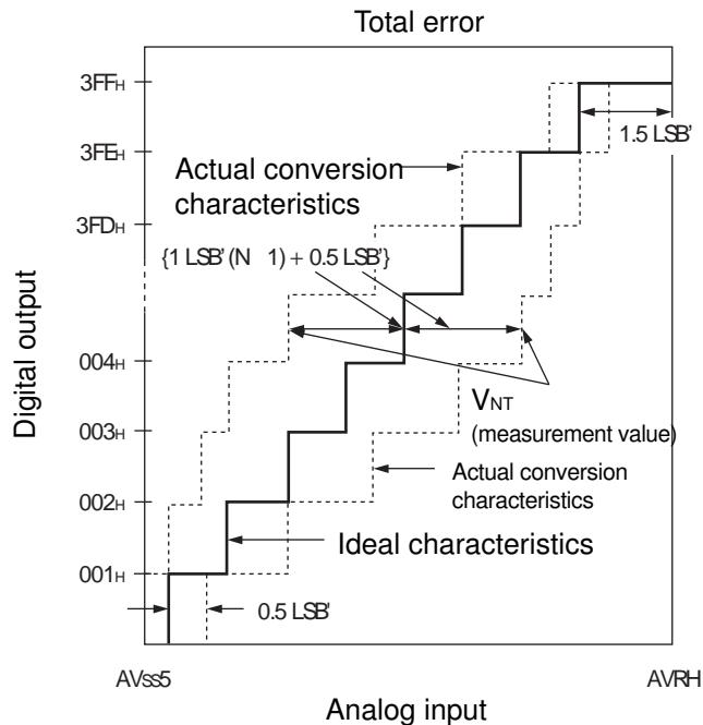
$$1 \text{ LSB}' (\text{ideal value}) = \frac{\text{AVRH} - \text{AVss5}}{1024} [\text{V}]$$
