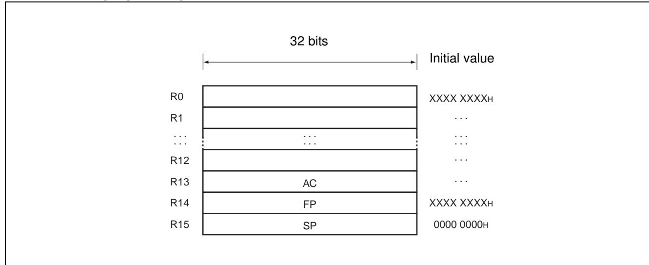
Registers R0 to R15 are general-purpose registers. These registers can be used as accumulators for computation operations and as pointers for memory access.
