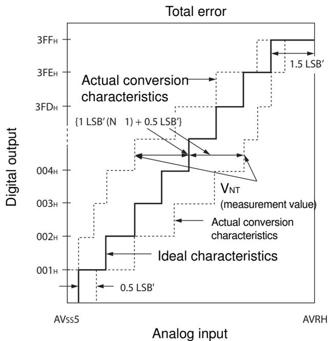
$$1\text{LSB}' \text{ (ideal value)} = \frac{\text{AV}_{\text{RH}} - \text{AV}_{\text{SS5}}}{1024} \text{ [V]}$$
