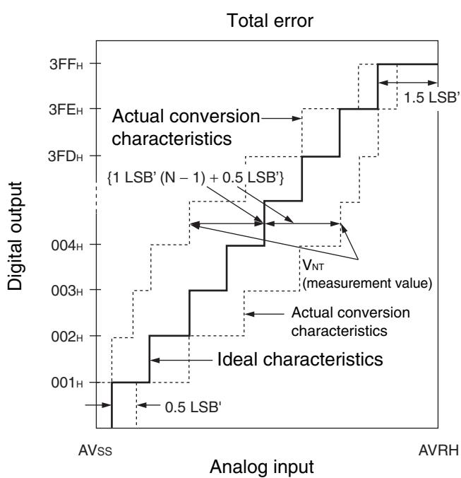
$$1\text{LSB}' (\text{ideal value}) = \frac{\text{AVRH} - \text{AV}_{\text{ss}}}{1024} [\text{V}]$$
