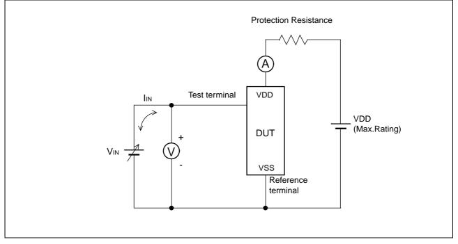
Note : The voltage V<sub>IN</sub> is increased gradually and the current I<sub>IN</sub> of 300 mA at maximum shall flow. Confirm the latch up does not occur under I<sub>IN</sub> = ± 300 mA. In case the specific requirement is specified for I/O and I<sub>IN</sub> cannot be 300 mA, the voltage shall be increased to the level that meets the specific requirement. • C-V method of Latch-Up Resistance Test
