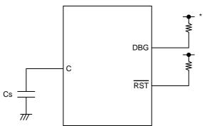
\*: Connect the DBG pin to an external pull-up resistor of 2 k $\Omega$  or above. After power-on, ensure that the DBG pin does not stay at "L" level until the reset output is released. The DBG pin becomes a communication pin in debug mode. Since the actual pull-up resistance depends on the tool used and the interconnection length, refer to the tool document when selecting a pull-up resistor.
