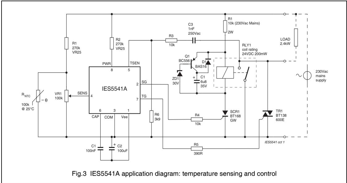
Fig.3 IES5541A application diagram: temperature sensing and control
