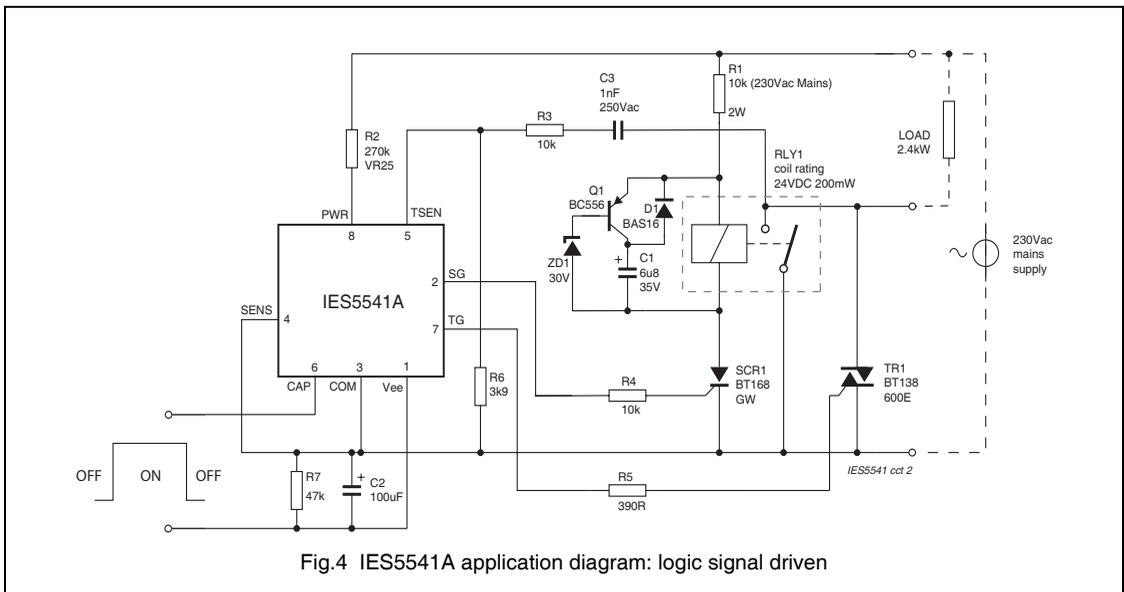
Fig.4 IES5541A application diagram: logic signal driven
