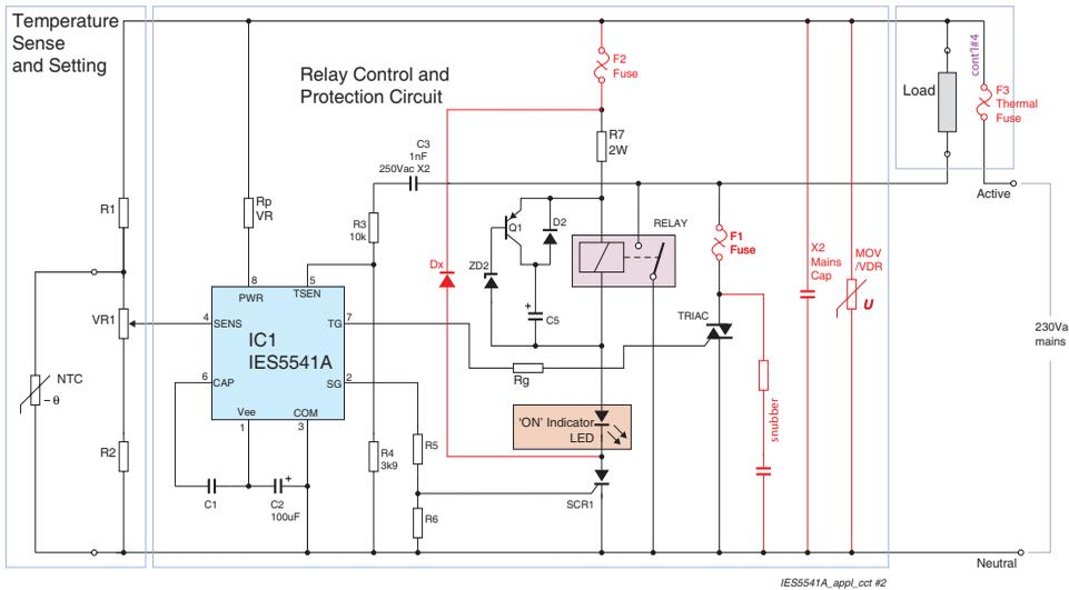
Fig.7 IES5541A application diagram:
