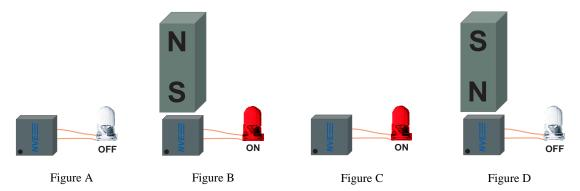
As a south magnetic field is applied to the pin 8 side of the sensor, the digital output will turn on (Figure B). A north magnetic field applied to the pin 1 side will also turn the output on. The output will remain latched on (Figure C) until an opposite field is applied (Figure D).
