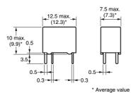
Note: Each value has a tolerance of ±0.3 mm.
