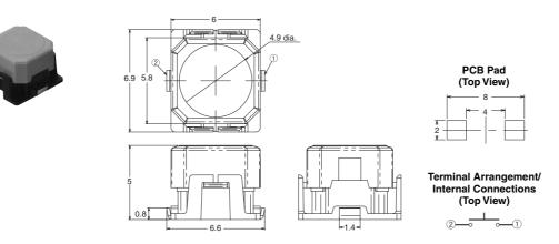
Note: Unless otherwise specified, a tolerance of  $\pm 0.4$  mm applies to all dimensions. No terminal numbers are indicated on the Switches.
