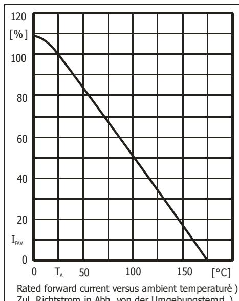
Rated forward current versus ambient temperature
