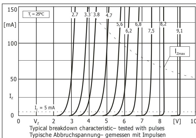
Typical breakdown characteristic - tested with pulses
