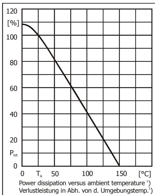
1 Valid, if leads are kept at ambient temperature at a distance of 2 mm from case
