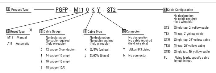
1. Manual configuration should be specified if automatic power-up, after power restoration of circuit power, could create an unsafe condition.
