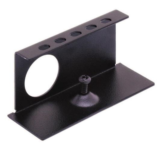
The FP-CT1 is a mounting bracket that fits the mounting track on FP-RRA and FP-RRAH rack mount panels. The set screw allows the installer to secure the bracket into position. An FP-CT1 can be secured at each end of an installed FLAT-PAK module, thereby securing the FLAT-PAK in mobile installations. Slots in the front surface of the bracket allow the installer to secure wires and cables in place. The FLAT-PAK power interconnect cables may be installed through the FP-CT1.
