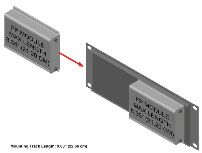
Required mounting length for multiple modules is the module length plus .65 in (1.65 cm) for each power interconnection.
