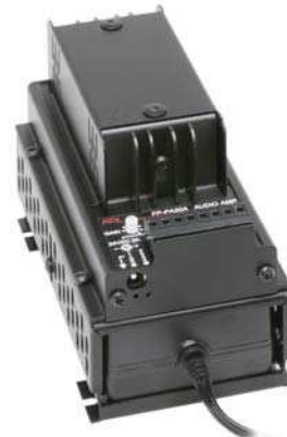
FP-PSB1A with power supply and FP-PA20 audio amplifier mounted
