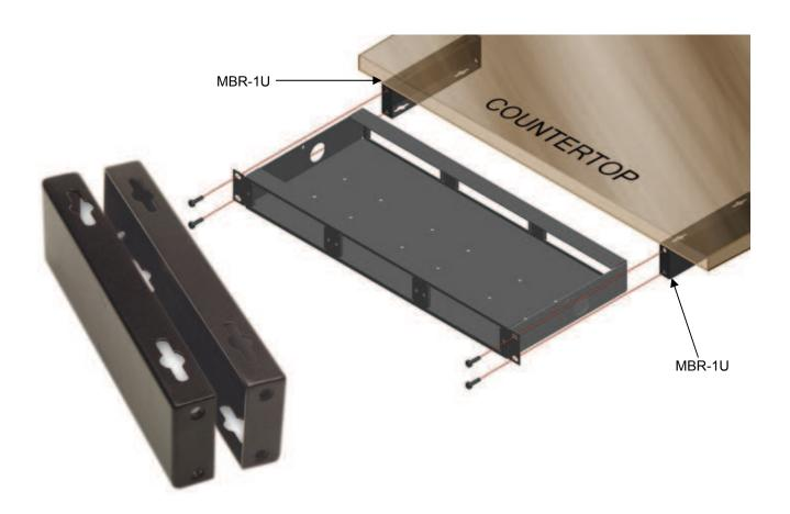
The MBR-1U mounting kit contains two brackets designed to mount to any flat surface or under a shelf. The brackets hold standard 19" rack mounted equipment 1RU in height. Threads for either US #10-32 or metric M5 rack screws are provided. The MBR-1U is ideal for mounting RDL racking accessories and many 1RU industry products.
