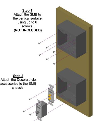
The SMB-1, 2, 3 and 4 surface mount boxes hold one, two, three or four Decora®-style products, including RDL remote controls and connector plates.
