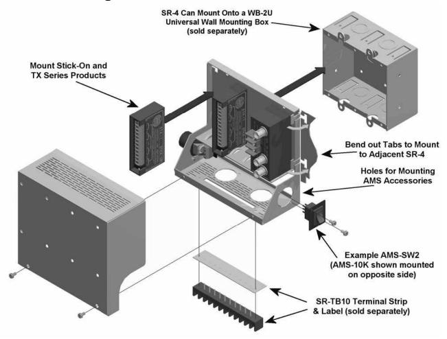
Mounting holes in the SR-4 permit attachment in a variety of locations, including cabinets, backboards, walls and plenums. The SR-4 holds up to 7 STICK-ONS. If power amplifier modules requiring convection cooling are mounted, a maximum of 4 should be installed, leaving an empty space between modules. 7 STICK-ONS may be mounted if they are not heat generating modules. TX<sup>™</sup> modules will also fit in the SR-4.
