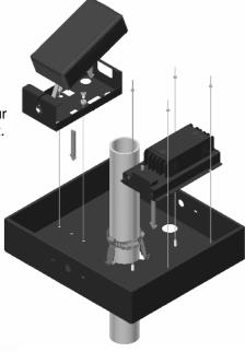
2. Secure the tray by tightening the hose clamp to mounting brackets using a screwdriver.
