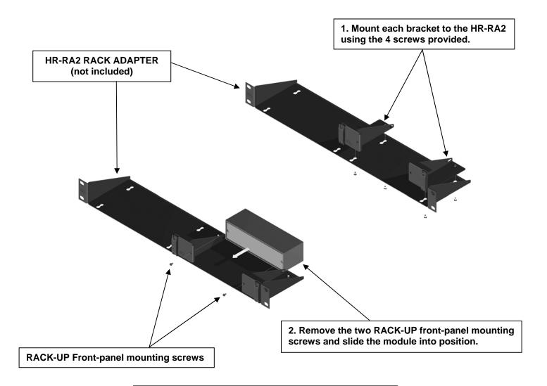
3. Fasten the RACK-UP module to the HR-RU1 brackets using the module front-panel mounting screws.
