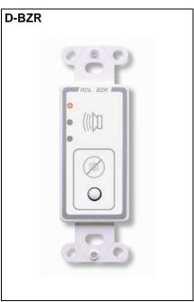
The BZR power supply input accepts 24 Volts *ac* or *dc*. The BZR is a negative ground-referenced product. In the unlikely event it is connected on a common 24 Vac supply together with equipment which is positive ground-referenced *and* not transformer isolated, a ground fault may occur. The BZR automatically detects such a fault and disconnects itself from the power input.
