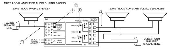
PAGING SIGNAL MUTES ZONE / ROOM AMPLIFIED PROGRAM SOURCE WHEN PAGE IS PRESENT NOTE: THE PAGING SOURCE AND LOCAL AMPLIFIER MUST BE SET TO THE SAME CONSTANT VOLTAGE (25 V, 70 V OR 100 V)
