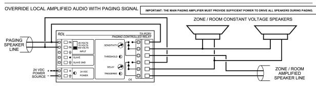
PAGING SIGNAL OVERRIDES ZONE/ROOM AMPLIFIED PROGRAM SOURCE WHEN PAGE IS PRESENT NOTE: THE PAGING SOURCE AND LOCAL AMPLIFIER MUST BE SET TO THE SAME CONSTANT VOLTAGE (25 V, 70 V OR 100 V)
