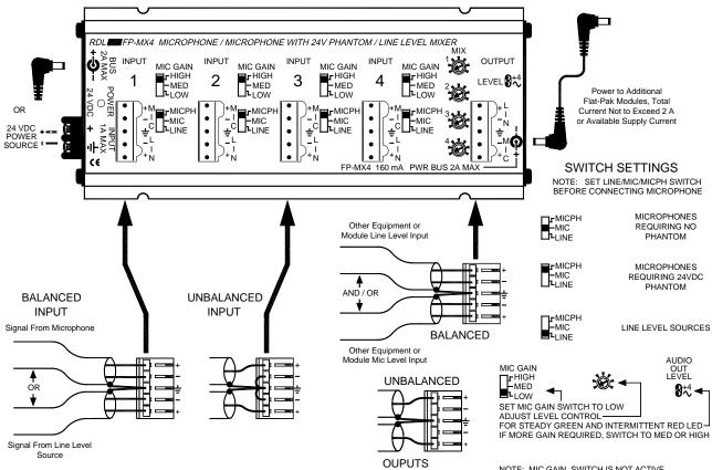
EACH INPUT OR OUTPUT MAY BE WIRED BALANCED OR UNBALANCED
