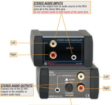
**GROUND-LIFT SWITCH**The audio output cable shields are connected to the EZ-HK1 chassis when the switch is in the NORM position. In the unlikely event that the EZ-HK1 chassis is mounted to equipment with a different ground from the equipment the EZ-HK1 output is feeding, a ground loop could be produced. This ground loop is eliminated by setting the switch to the LIFT position.
