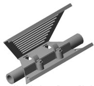
Install bracket to pipe or tubing using the smallest possible clamp provided. The clamp must be oriented as shown with the "tail" inside the bracket.
