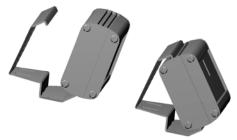
Secure the unit in the mounting bracket: •First, seat the bottom bracket in the SAS-HC8 bottom rear slot;
