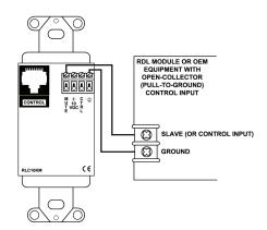
Note: The **MUTE** output terminal is pulled to ground when the module is set to mute. Connections to this terminal do not affect the proper operation of the VCA control output.
