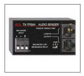
The TX-TPS6A is a single-pair audio sending module compatible with RDL Format-A twisted pair products. It is built in the versatile Max-TX series enclosure. The durable adhesives provided with the TX-TPS6A permit permanent or removable mounting. The TX-TPS6A may be rack or surface mounted with optional TX™ series accessories.
