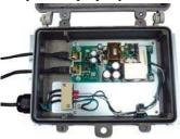
7) Reattach the protective covering over the PC board and terminal blocks and re-close the lid. Ensure that the four captive screws are fully tightened before operation can commence.
