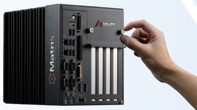
1. Undo the thumbscrews by hand
