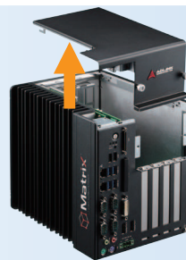
2. Withdraw the thumbscrew and remove the top cover
