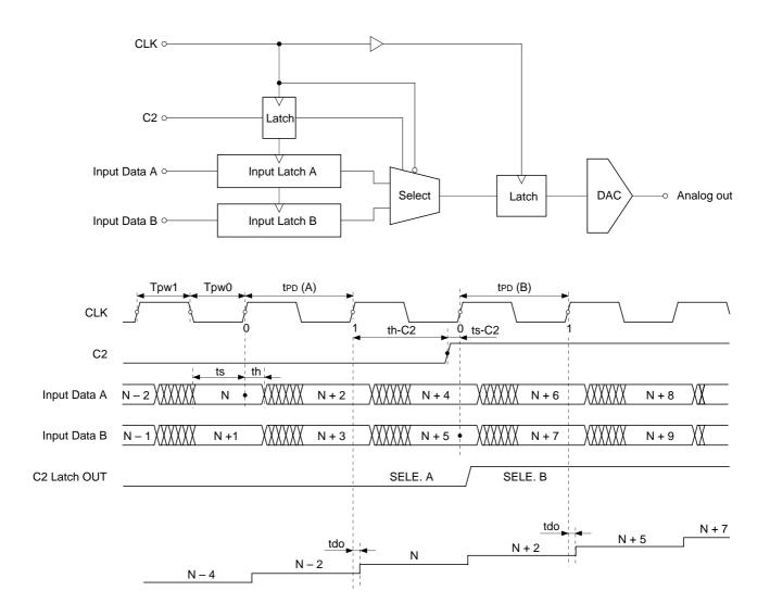
In SELE.A and SELE.B modes, input Data A or Data B is selected and the selected data can be analog output. When C1 = 1 and C3 = 0, Data A is selected for C2 = 0, and Data B is selected for C2 = 1.
