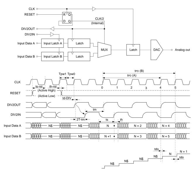
In MUX.1A mode, Data A and Data B are internally multiplexed and then the resulting signal can be analog output. The frequency of the clock is halved by the built-in clock frequency divider circuit and the CLK/2 can be output at TTL level (DIV2OUT). CLK/2 can be reset by the reset signal.
