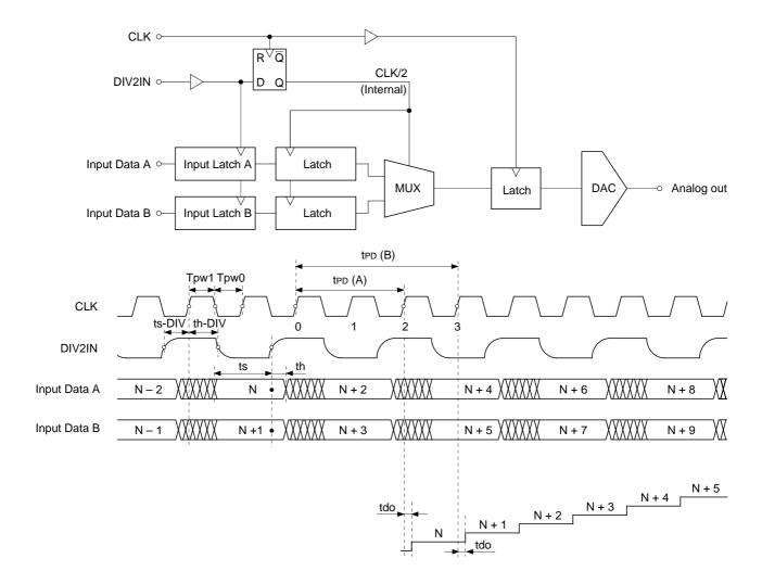
In MUX.2 mode, the 1/2 frequency-divided clock signal (DIV2IN) and Data A and Data B, which are synchronized with DIV2IN, are provided simultaneously. These signals are internally multiplexed and the resulting signal can be analog output.
