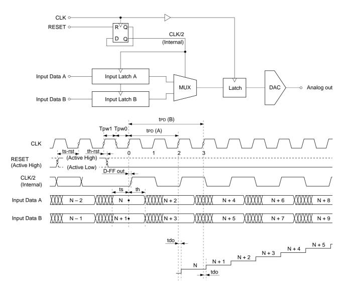
In MUX.1B mode, Data A and Data B are internally multiplexed and then the resulting signal can be analog output. The frequency of the clock is halved by the built-in clock frequency divider circuit. CLK/2 can be reset by the reset signal.
