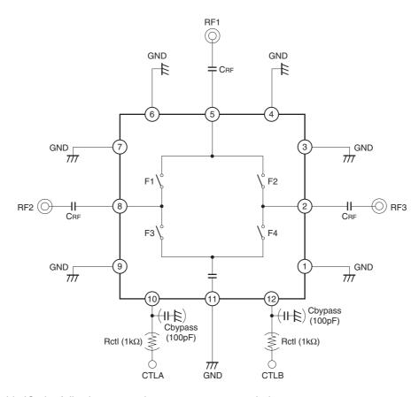
When using this IC, the following external components are needed:
