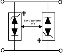
Application Note: Device must be used with two units in parallel,opposite in polarity as shown in circuit for AC signal line protection.
