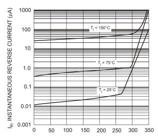
V<sub>R</sub>, INSTANTANEOUS REVERSE VOLTAGE (V) Fig. 3 Typical Reverse Characteristics, per element
