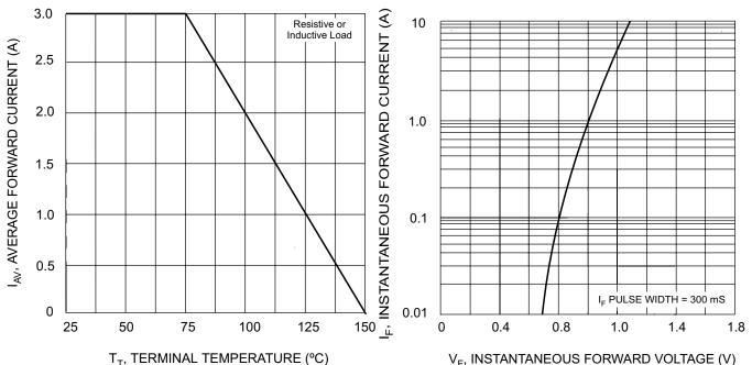
Fig. 1 Forward Current Derating Curve
