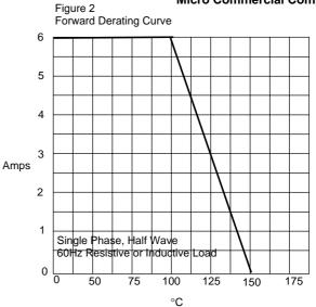
Average Forward Rectified Current - Amperes versus Ambient Temperature -  $^{\circ}\text{C}$
